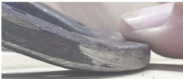
Above: Enhanced breakover of Rocker Toe.
