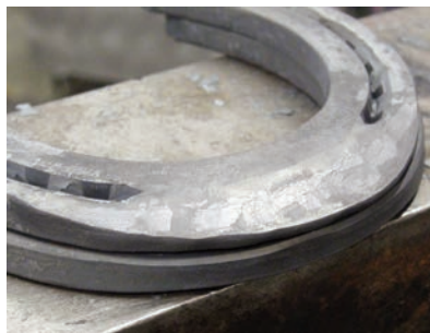
Rolled Toe before clean up.
