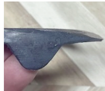
Lateral view of rolled toe.
