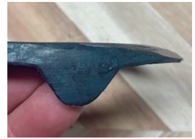
Lateral view of rolled toe.
