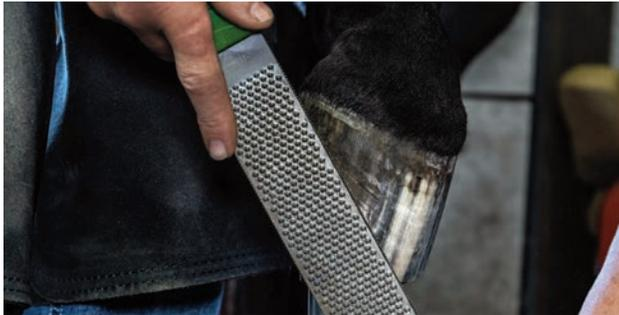
The innovative and unique manufacturing process of the Diamond Max Glide creates a high-quality rasp and file; 10% wider than the standard rasp. The rasp side features a 9-tooth pattern with slightly smaller teeth, and a file side with the chip breaker cut for a smooth finish.
