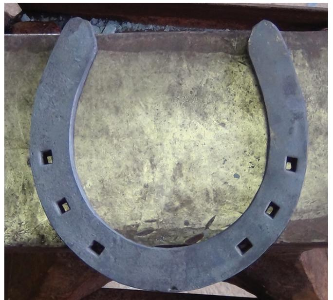
After drifting and pritcheling, make your flattening run and any last adjustments to shape.
