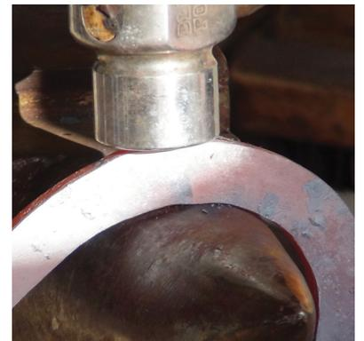
Turn branch over horn, striking the shoe just past the center of the horn to make the bend.
