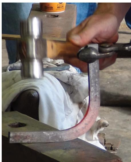
Working with round side of hammer, establish first one side of bend then the other.
